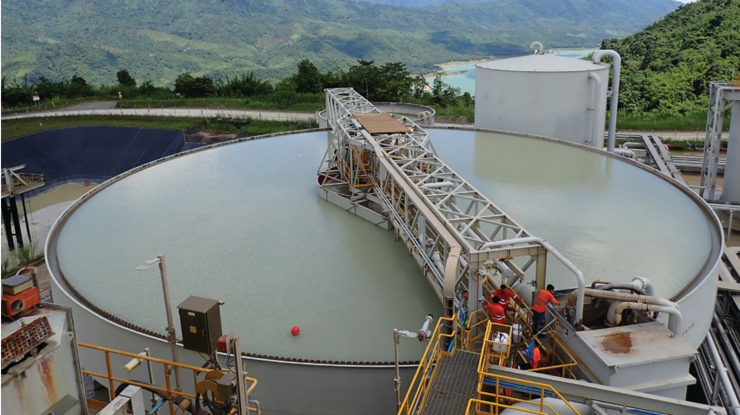
Upgrading key components of existing thickeners can improve performance and accommodate changes in duties and tailings characteristics at a much lower cost and downtime. Image: MINEXXT.
