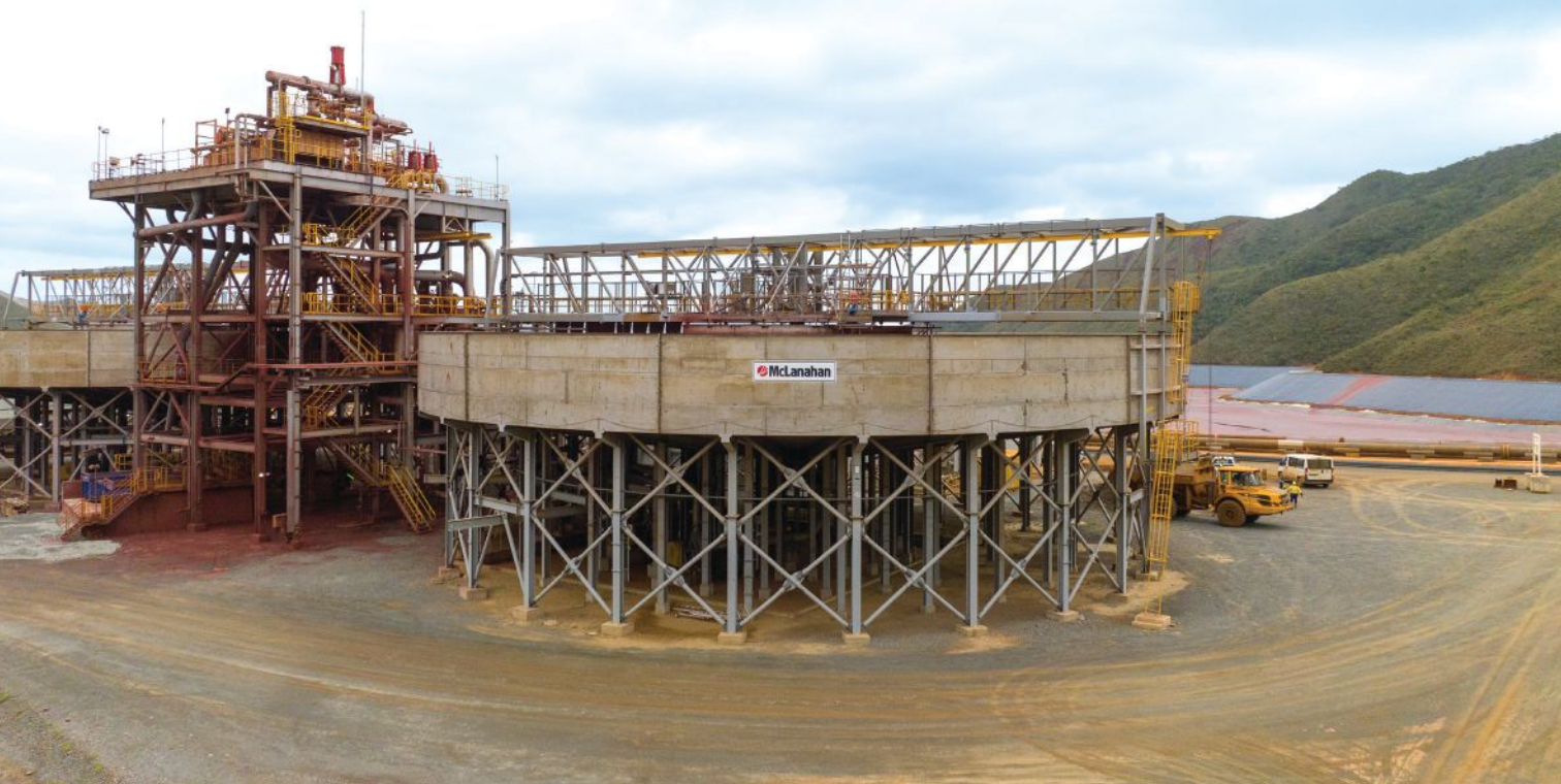
Thickeners employ chemical flocculation to separate liquid from solids. Clarified water is recovered from the overflow, while the thickened underflow is discharged for disposal or further dewatering. Pictured: A McLanahan thickener.
