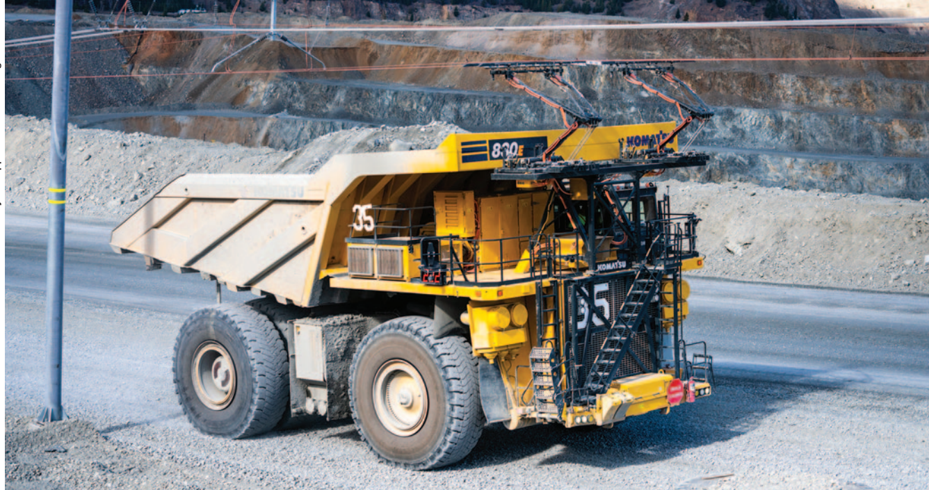
The Copper Mountain mine in British Columbia installed a trolley assist haul ramp, which allows electric haul trucks to climb the ramp at more than double the speed of diesel trucks.
